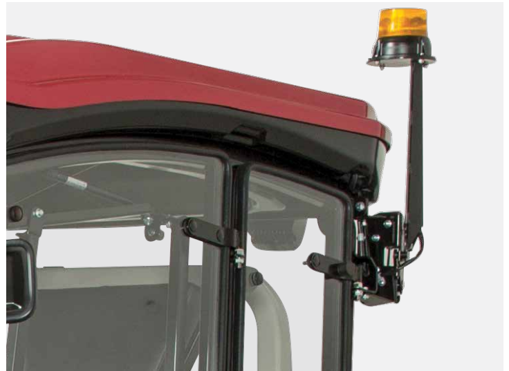
Fully Sealed, Breakaway Mounted Optional Strobe Beacon
